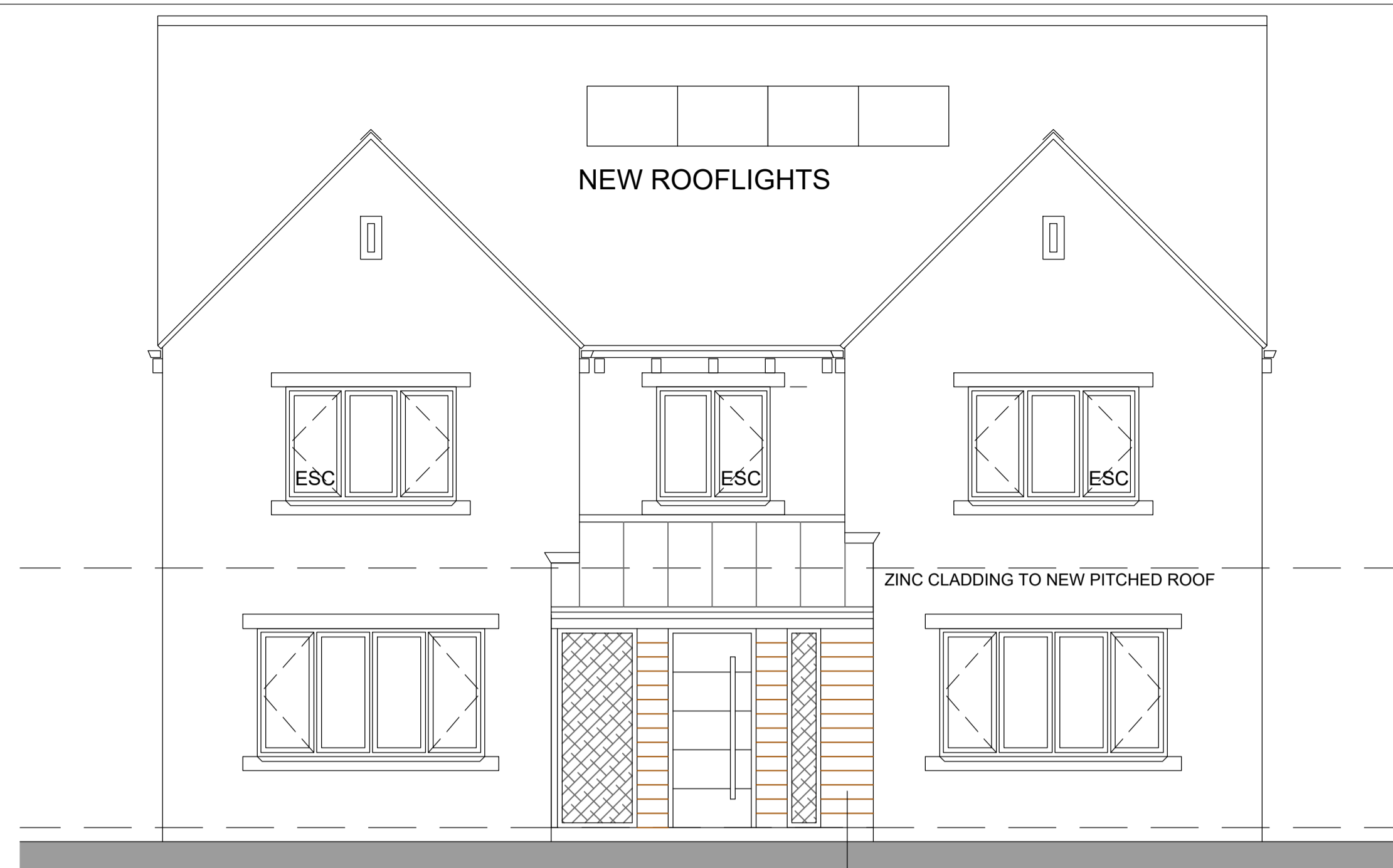
FRONT ELEVATION PROPOSED PORCH STONEMWORK TO MATCH EXISTING ALUMINIUM DOOR AND WINDOW FRAMES
