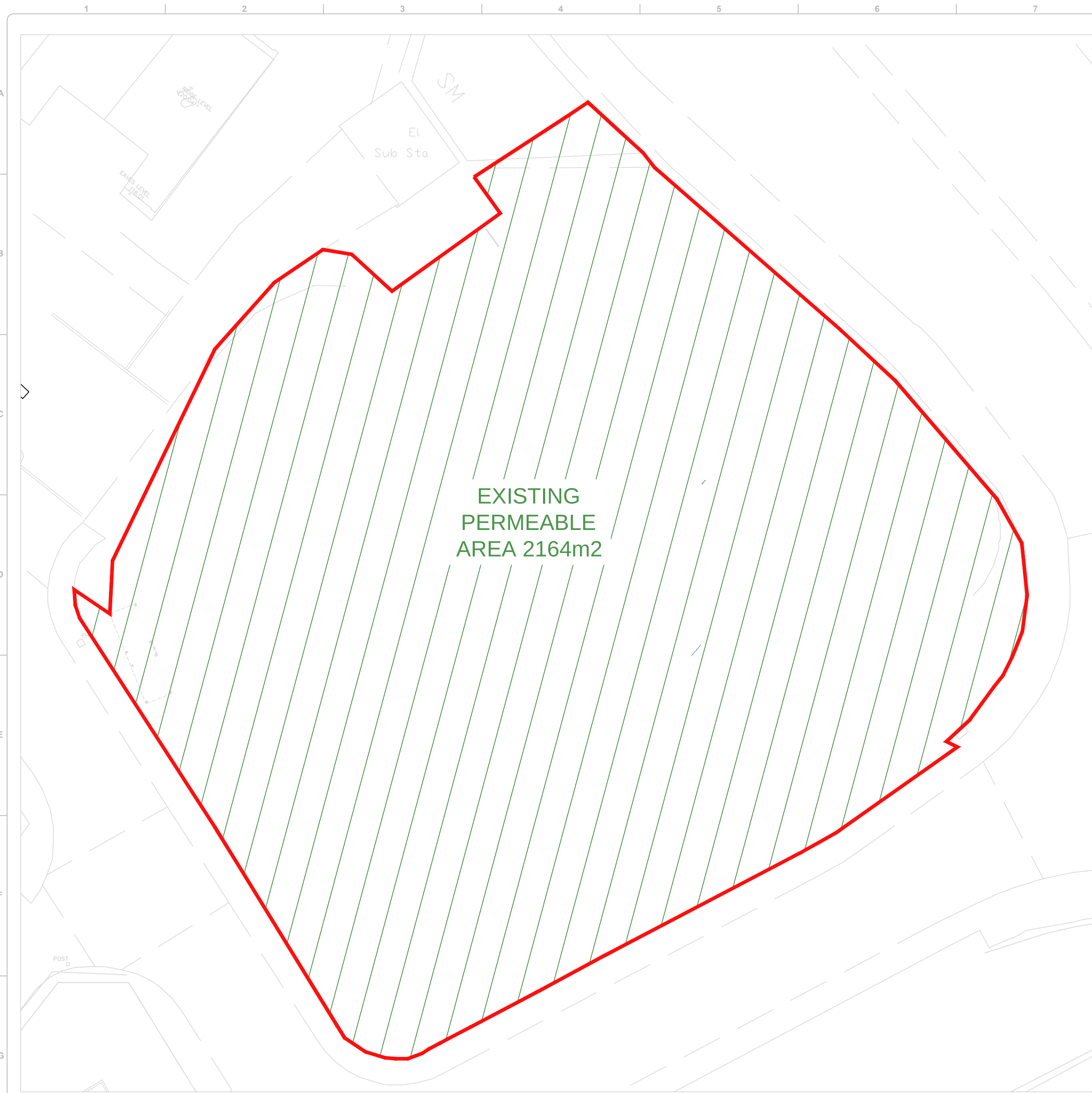
IMPERMEABLE/PERMEABLE AREAS (EXISTING) SCALE 1:200
