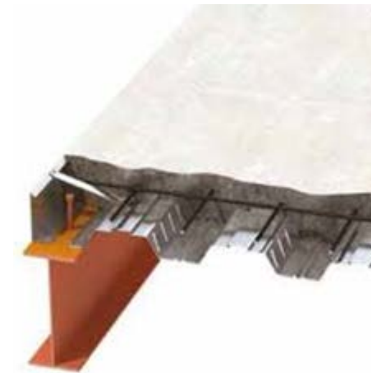
RC Slab on permanent metal decking construction
