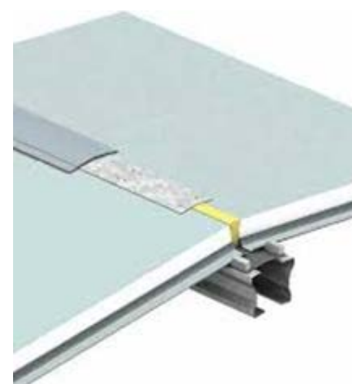
Kingspan Topdek panels supported on steel purlins
