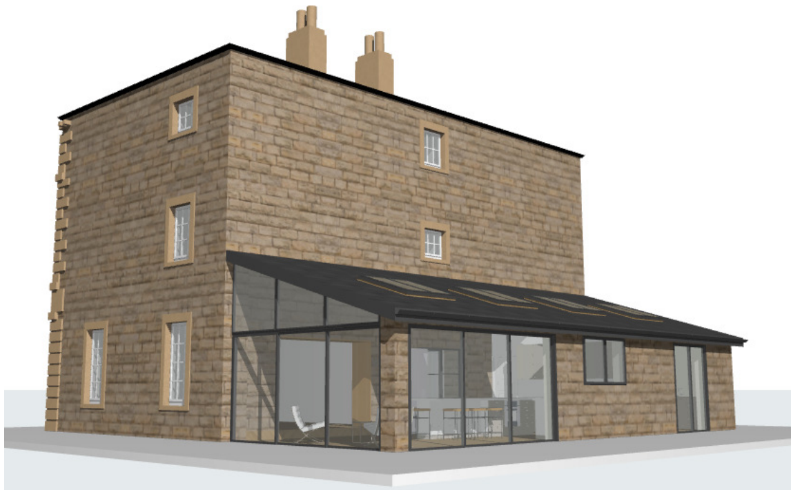
fig. 10 – Option 2 showing proposed materials with windows and doors in anthracite as a contrast to the stonework and to make the original materials and detailing stand out as the key heritage character.
