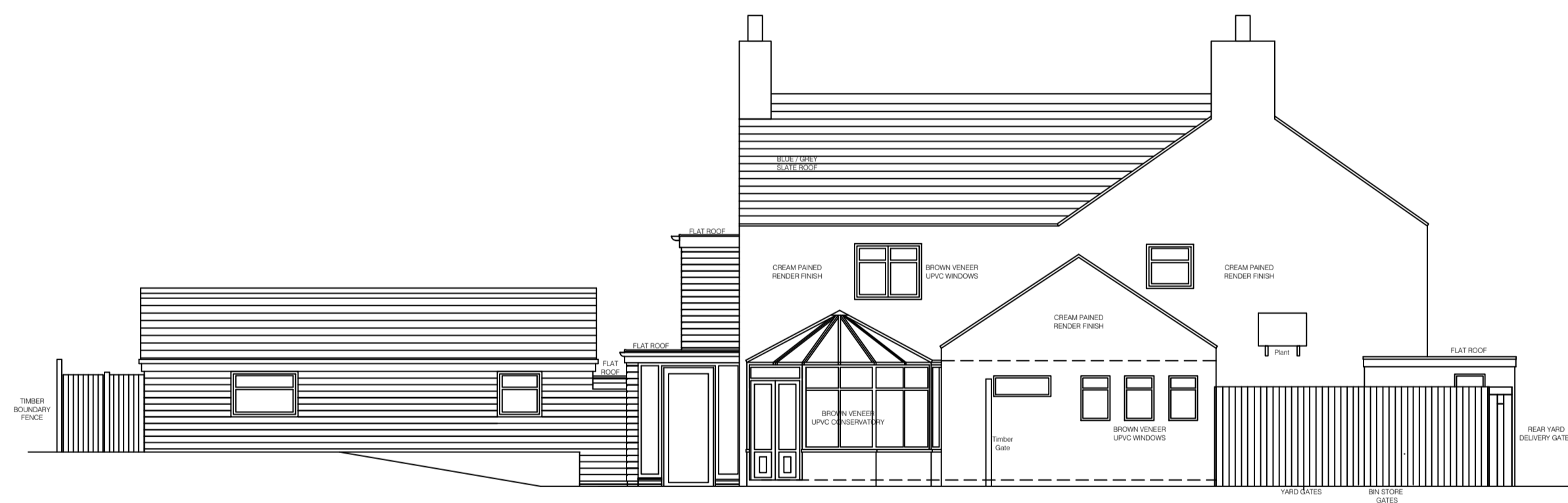
REAR ELEVATION AS EXISTING Scale: 1:100
