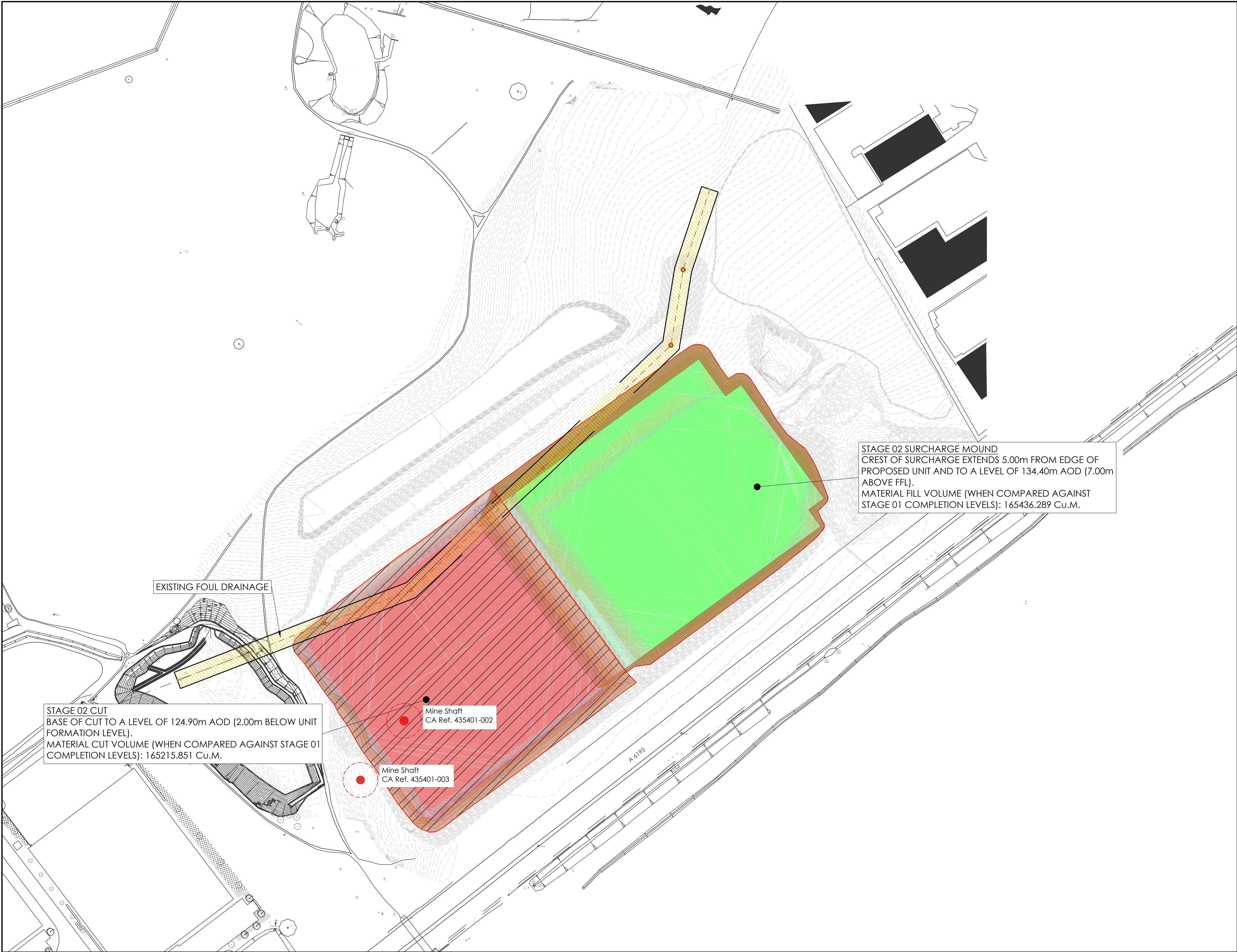
JPG-PROPOSED EARTHWORKS - STAGE 02 SCALE 1:1000
