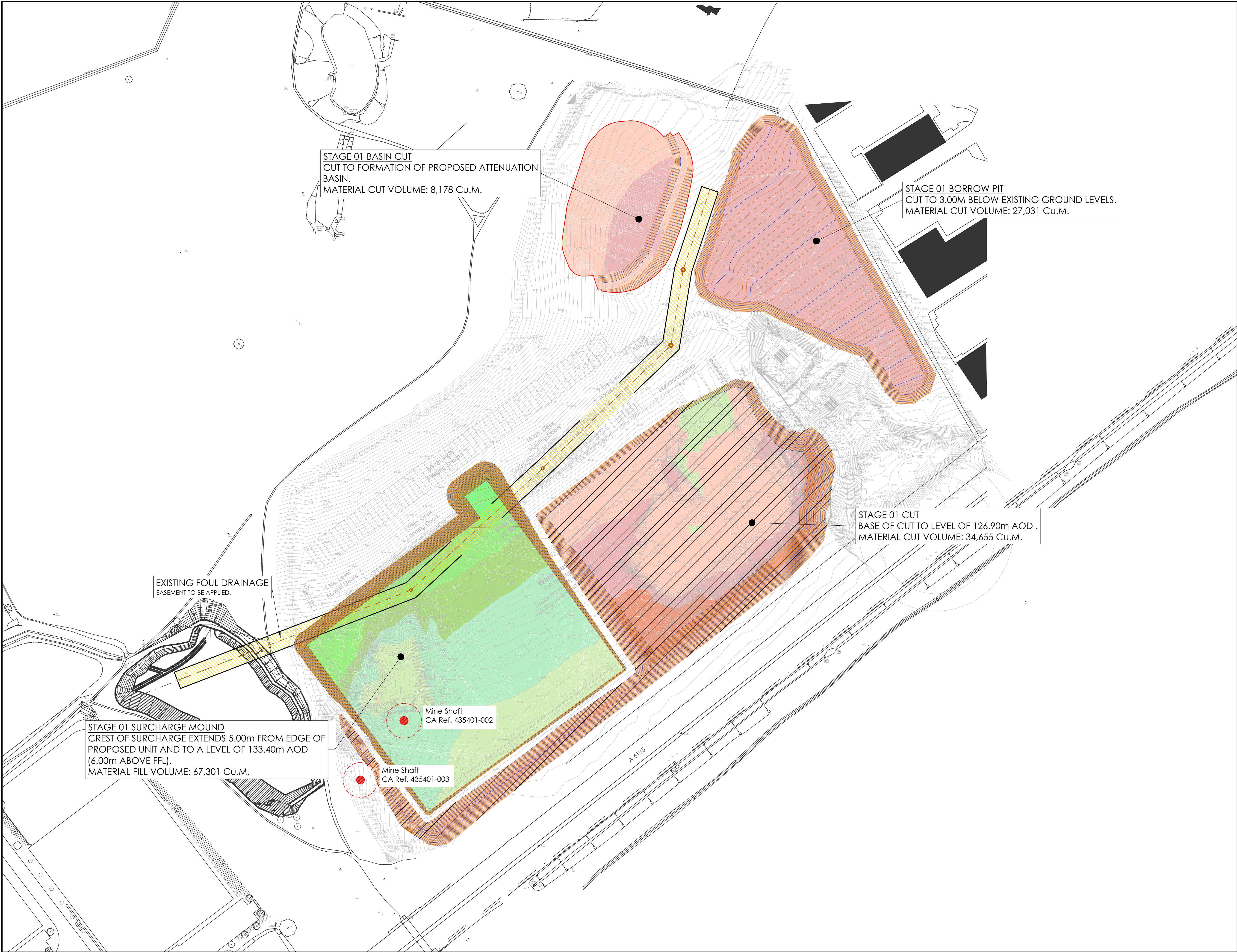
JPG-PROPOSED EARTHWORKS - STAGE 01 SCALE 1:1000
