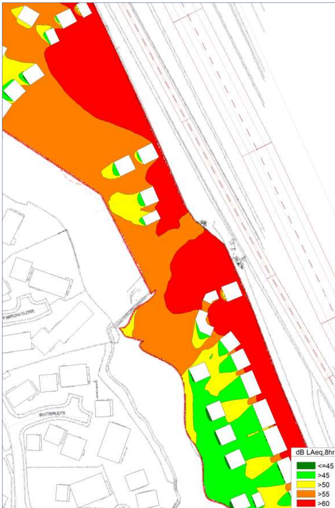
Figure C5: Night (Mid Part of Site) at 4m height
