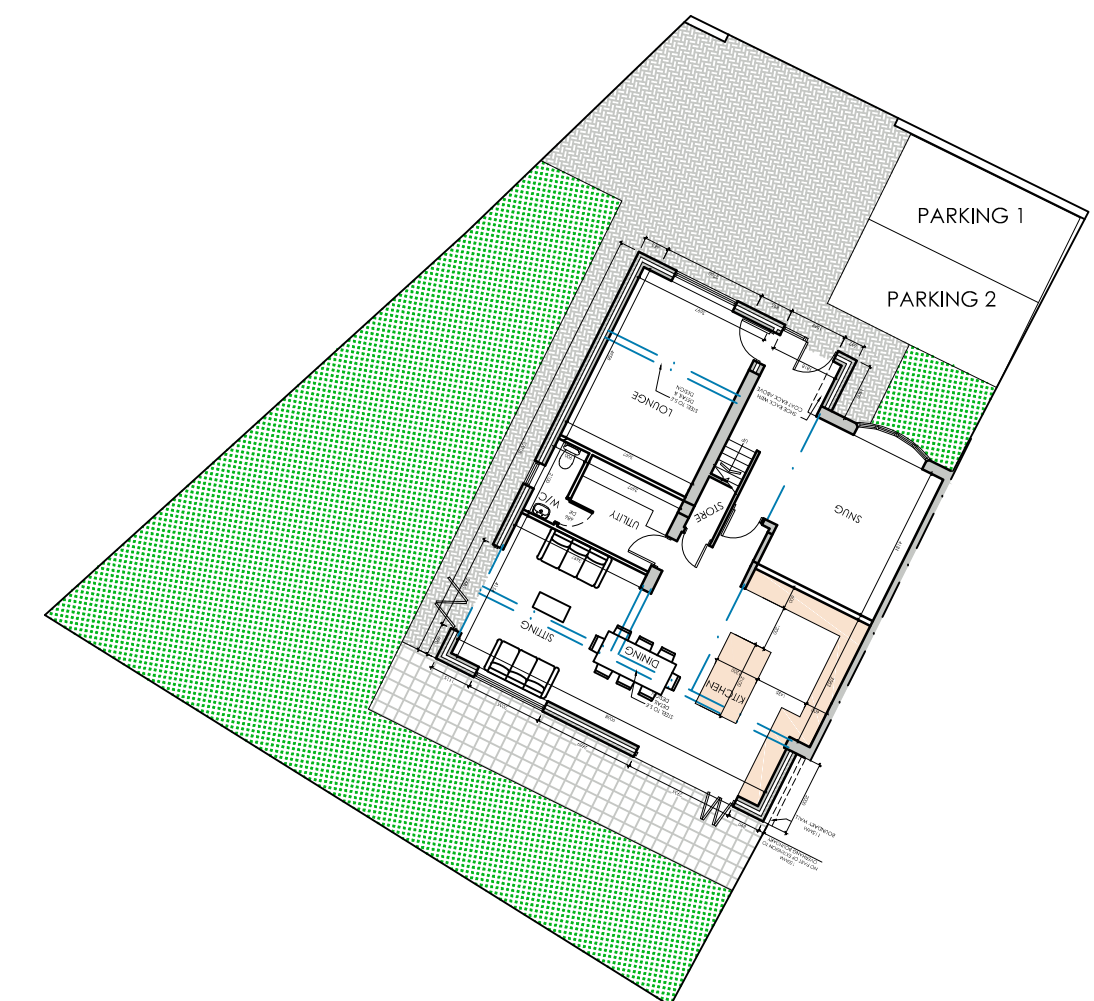
PROPOSED GROUND FLOOR WITHIN MEASURED SITE FOOTPRINT SCALE 1:200
