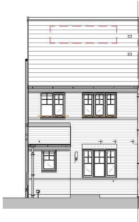
Front Elevation - Traditional Brick 1 : 100
