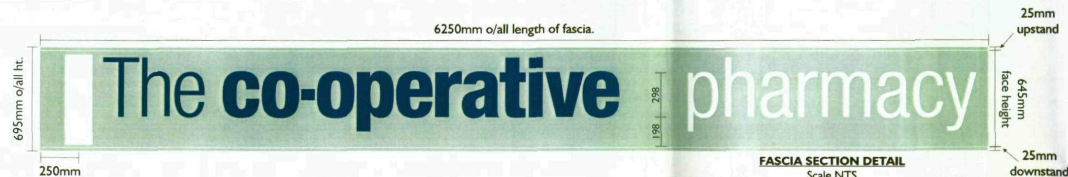
I OFF PART INTERNALLY ILLUMINATED FASCIA SIGN WITH M4 LETTERS - Scale 1:25
