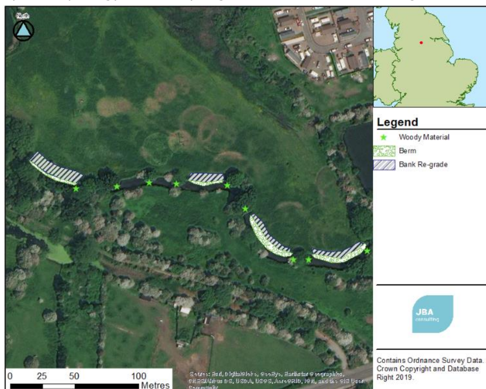
Figure 3-1: Proposed improvements for the downstream reach
