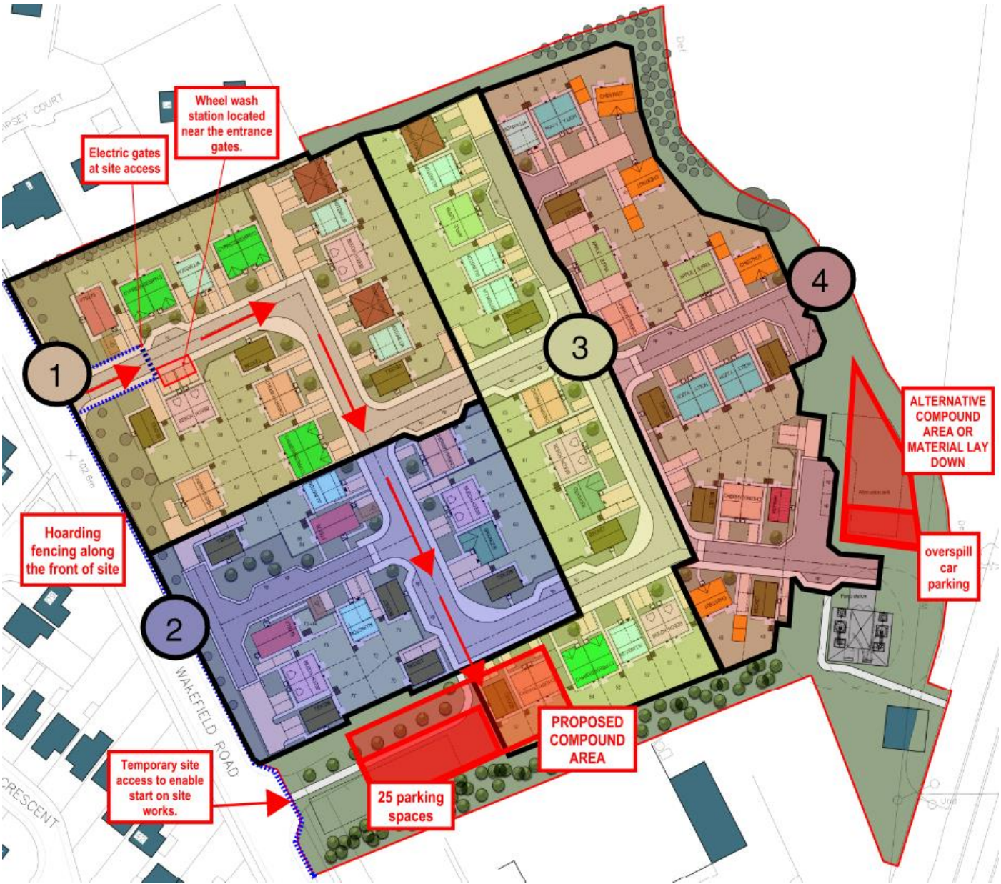
Figure 2. Construction Site Layout Plan.
