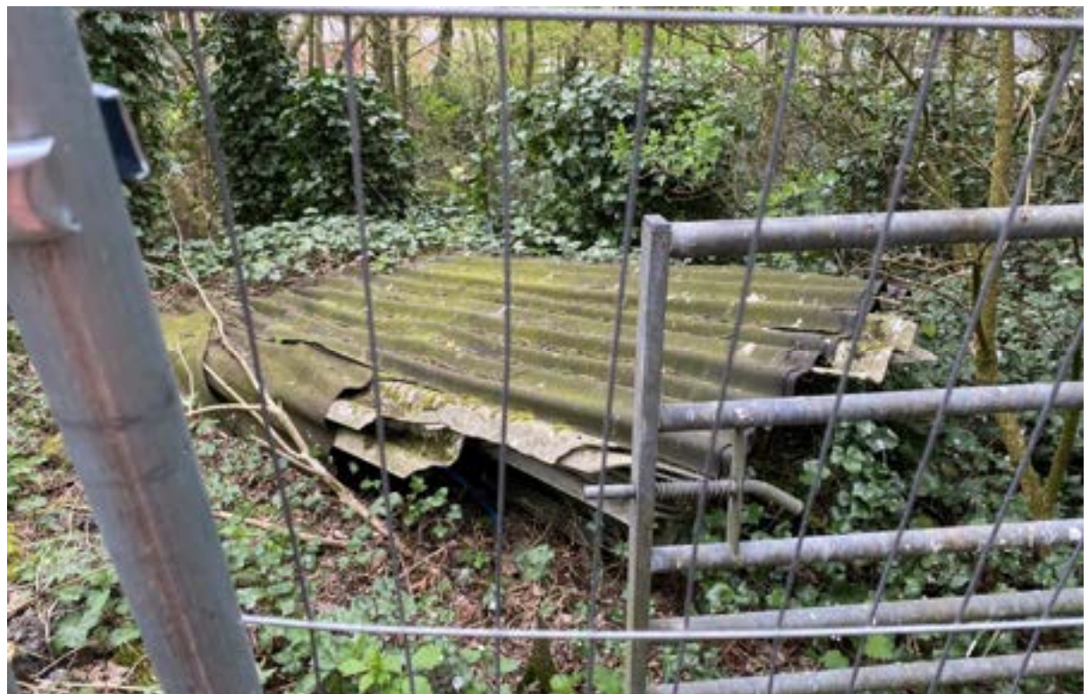
Photograph 4 – Stacked asbestos sheeting
