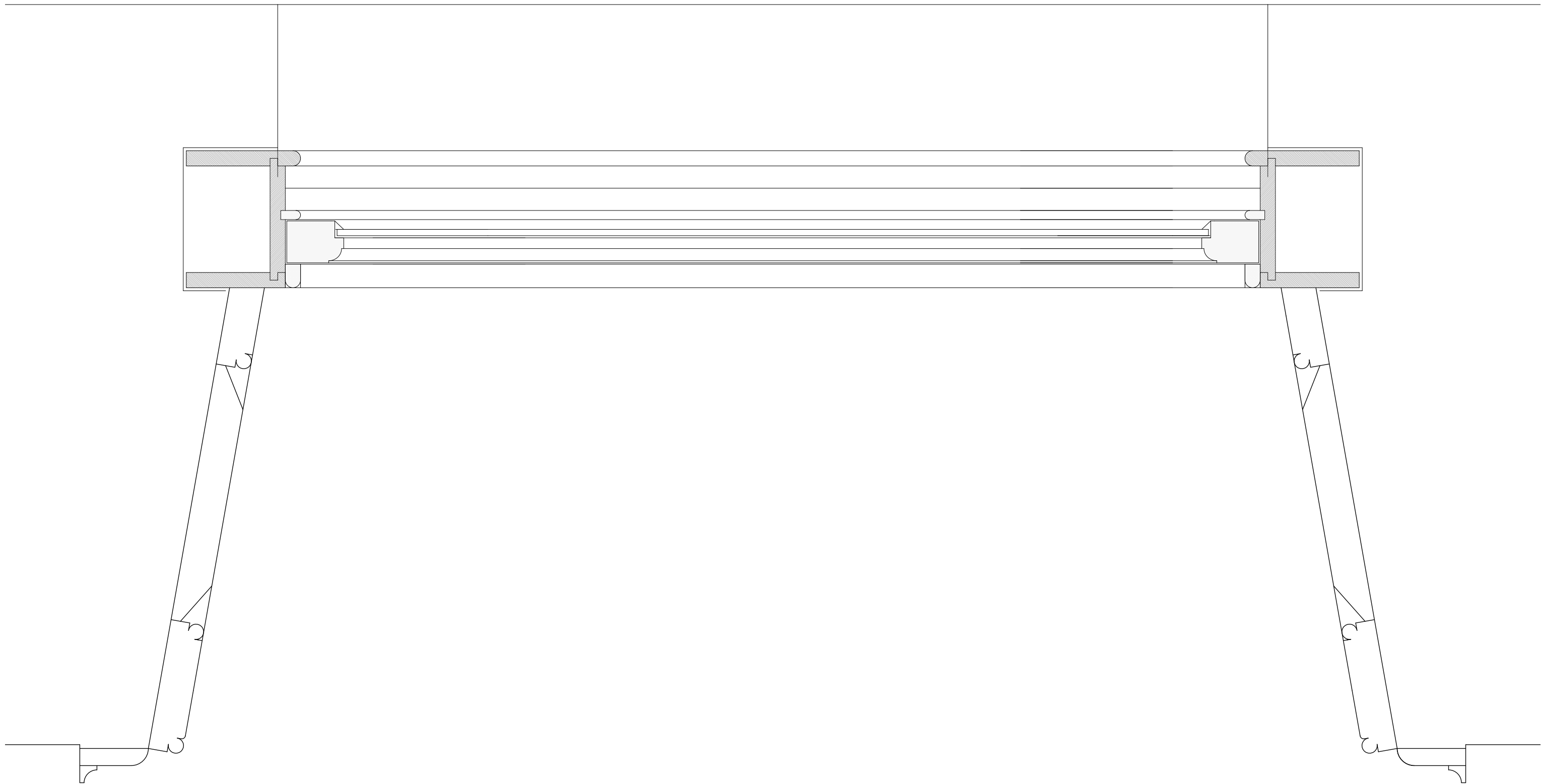
EXISTING WINDOW PLAN DETAIL SCALE 1:5
