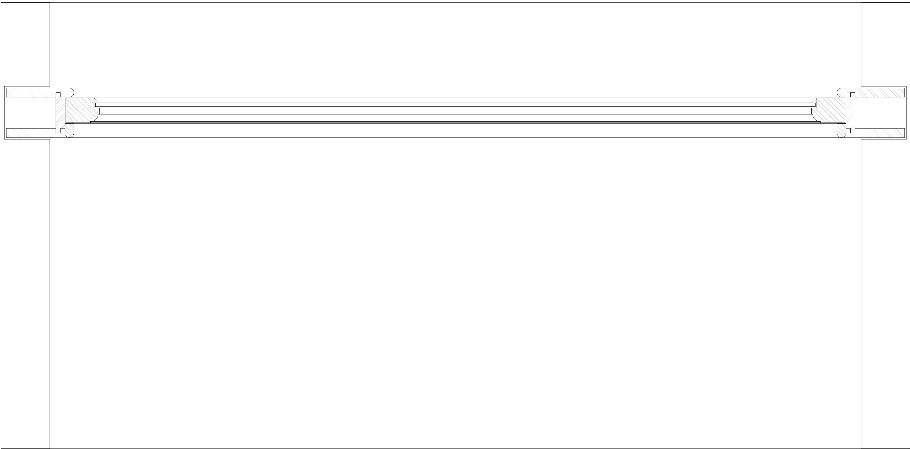
EXISTING WINDOW PLAN DETAIL SCALE 1:5
