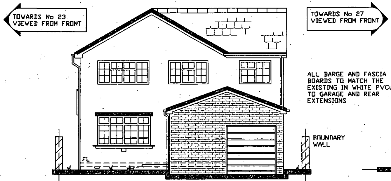
FRONT ELEVATION (FACING LONGSIDE WAY)
