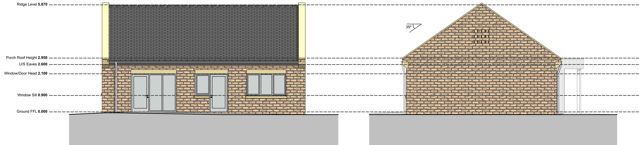
Bungalow Type 2B - Proposed Elevation C (Rear) - Scale 1:100
