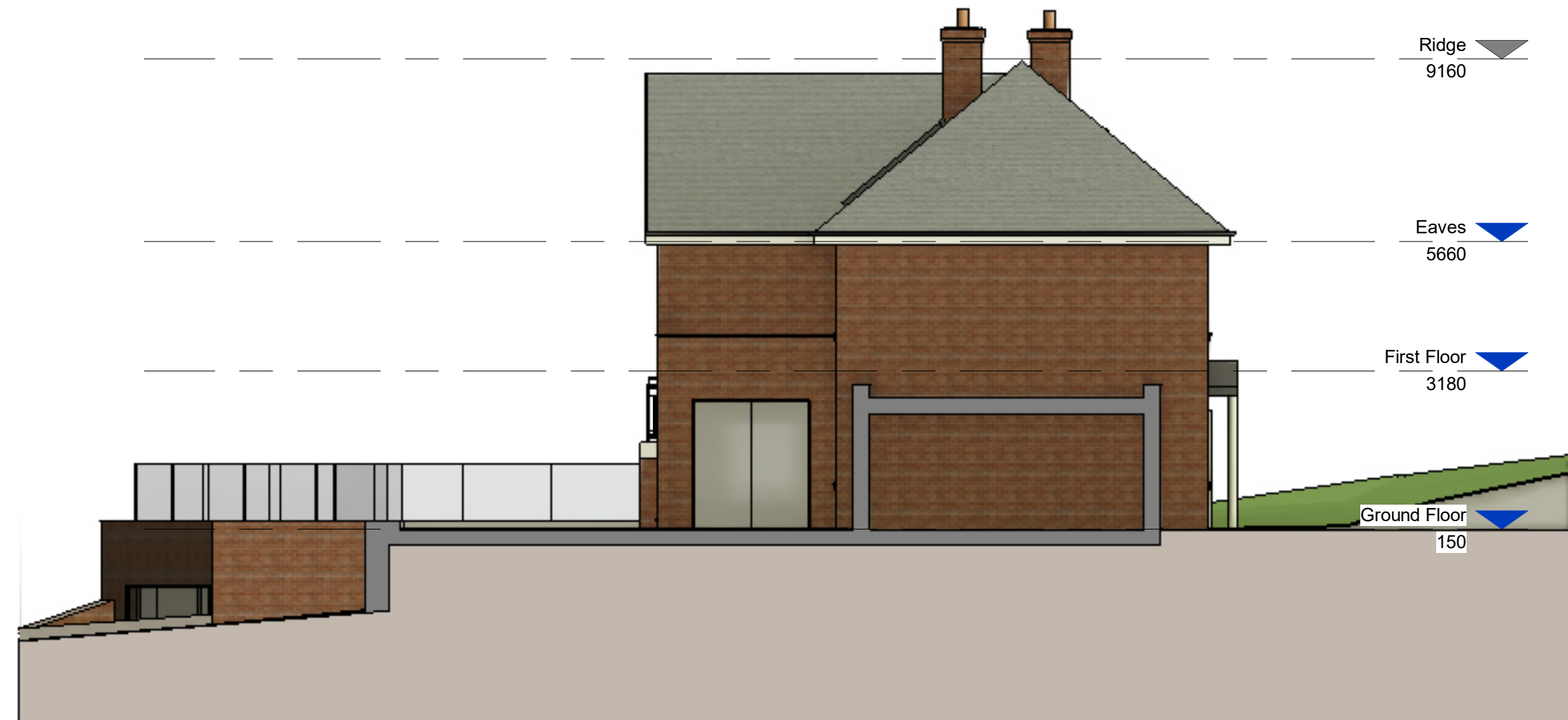
2 Proposed Side Elevation (South East) 1 : 100
