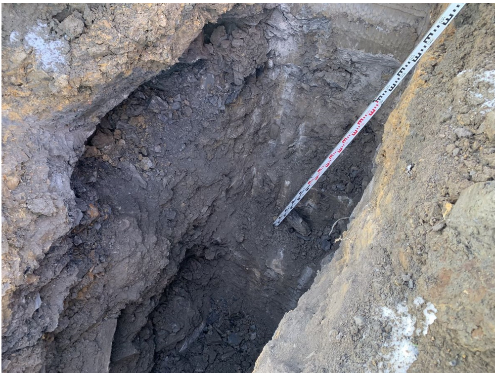
Photograph 39: Trial pit TP05. Stepped bedrock in north of trial pit, view from the south east to the north west.
