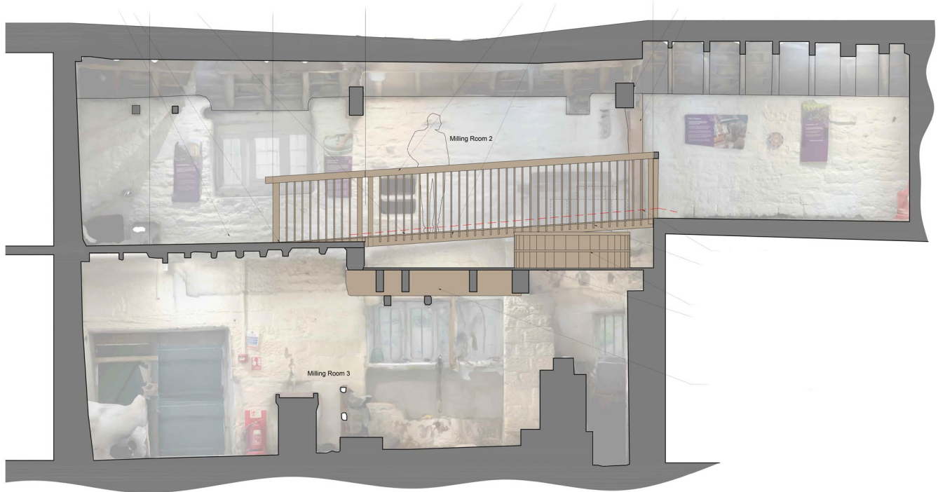
Figure 2: Section showing the proposed ramp.
