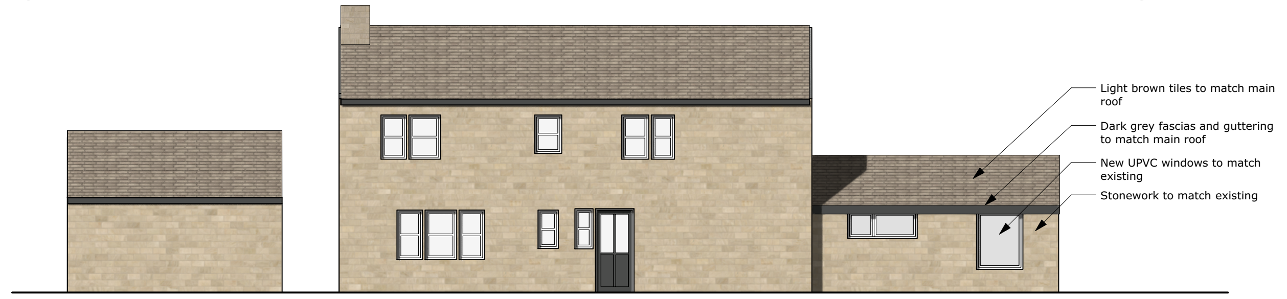
2 Proposed Rear Elevation Scale: 1:100
