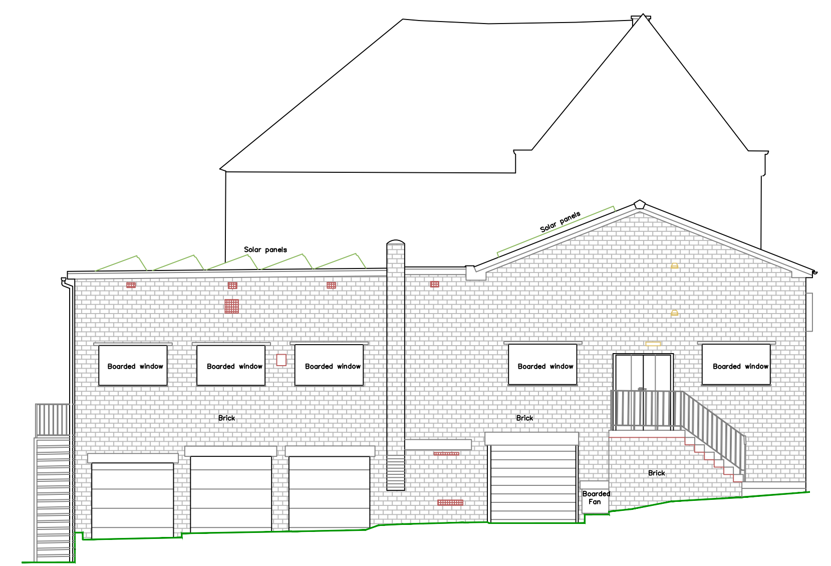
Existing Rear Elevation facing Brooke Street (East)
