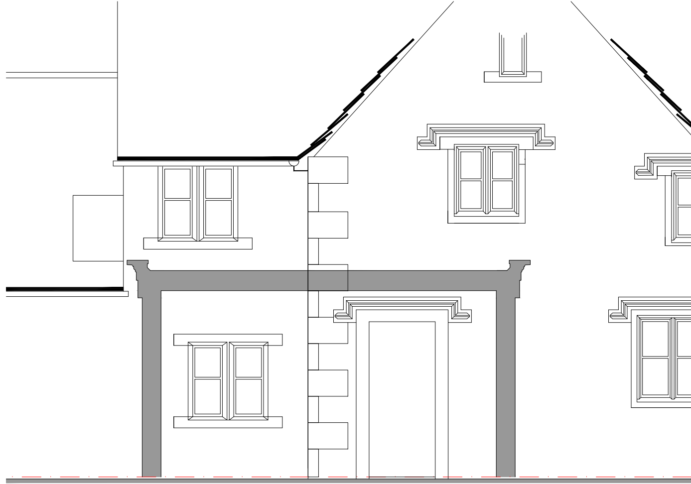
Elevation indicating connection to existing facade.
