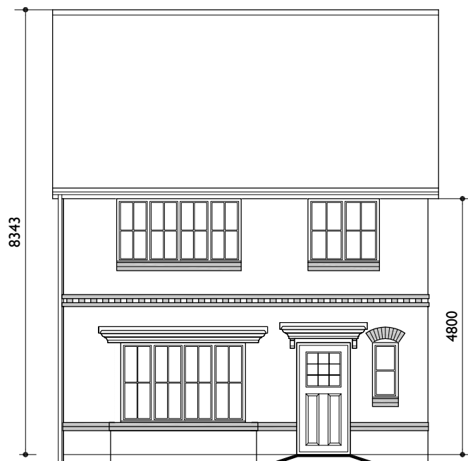
Front Elevation (Brick)
