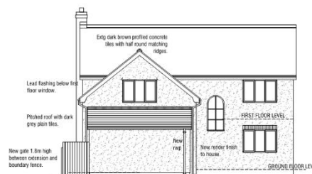
South West Elevation 1:100
