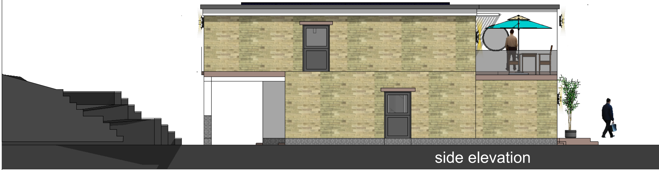
wienerberger Terca engineering brick blue perforated class B 65mm(or similar) below ground and up to DPC level with grey colour mortar
