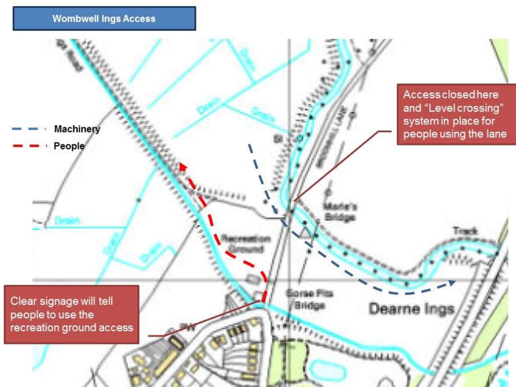
Figure 3-16 Access arrangements for Wombwell Ings during construction
