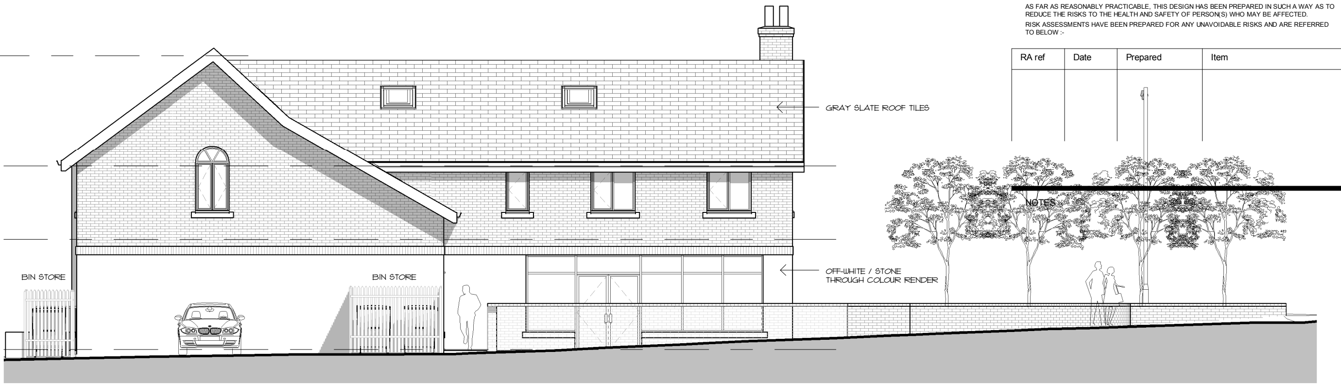
Rear Elevation (North Facing) 1 : 100
