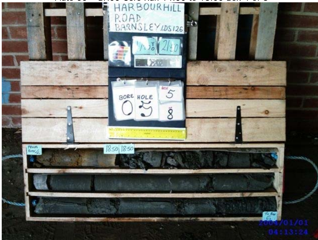
Plate 67 – BH05 Core Run 17.00 to 21.50 Box 5 of 8
