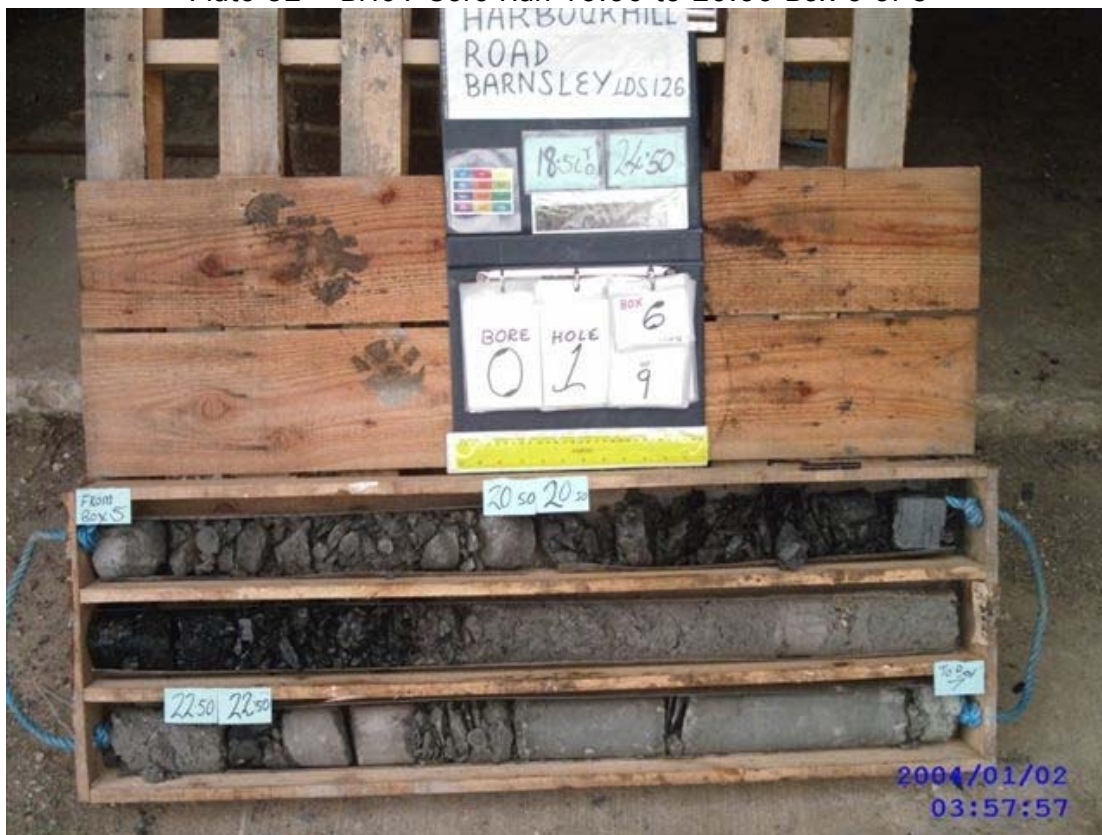
Plate 33 – BH01 Core run 18.50 to 24.50 Box 6 of 9
