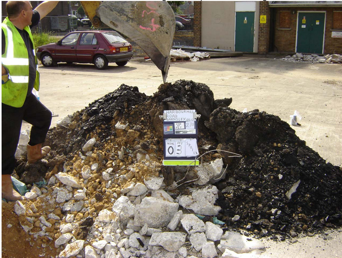
Plate 22 – Near surface coal extracted from Trial Pit 3
