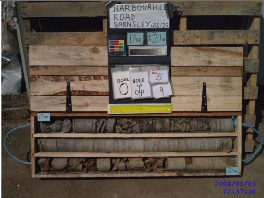
Plate 58 – BH04 Core Run 17.00 to 20.00 Box 5 of 9
