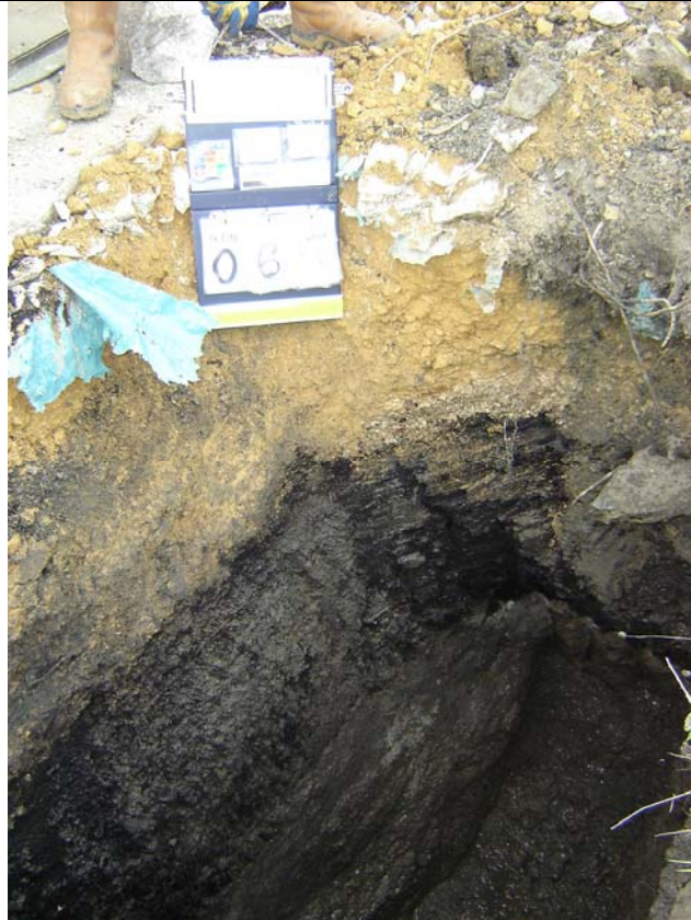
Plate 23 – Intact Coal in Trial Pit 6
