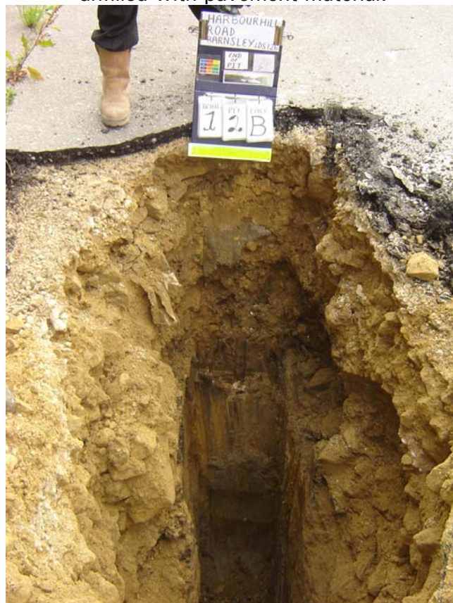
Plate 18 – Made ground of cobbles and boulders to 1.50m bgL and sandy gravelly clay to 2.00m bgL. This contained brick glass and fragments of polyethylene.
