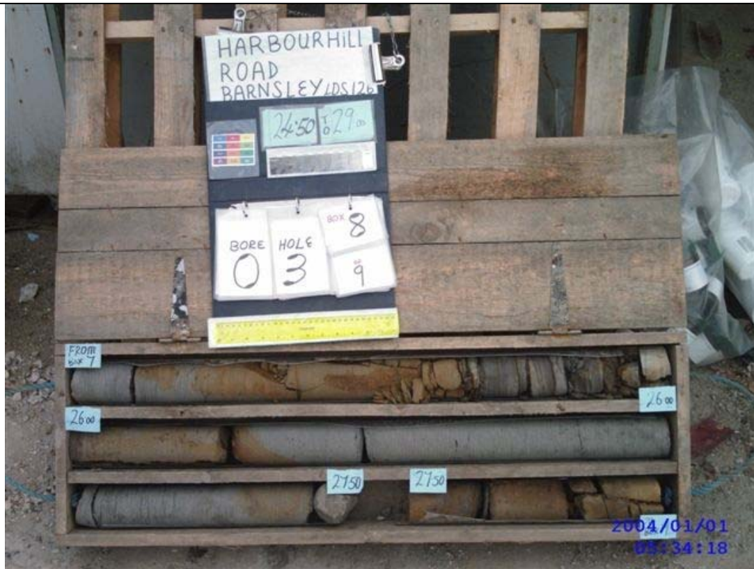
Plate 52 – BH03 Core Run 24.50 to 29.00 Box 8 of 9
