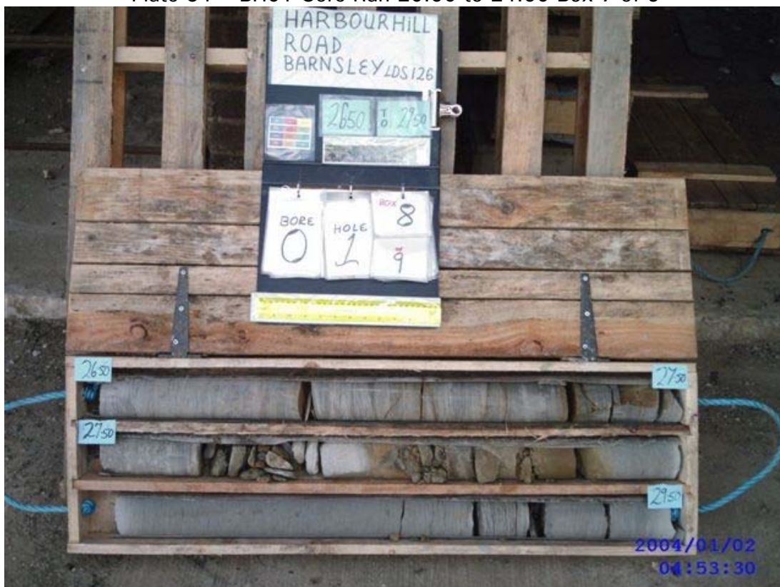
Plate 35 – BH01 Core Run 26.50 to 29.50 Box 8 of 9
