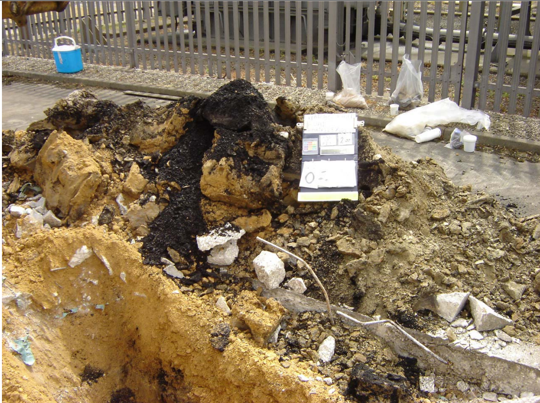
Plate 21 – Trial Pit 2 – Organic clay below made ground.
