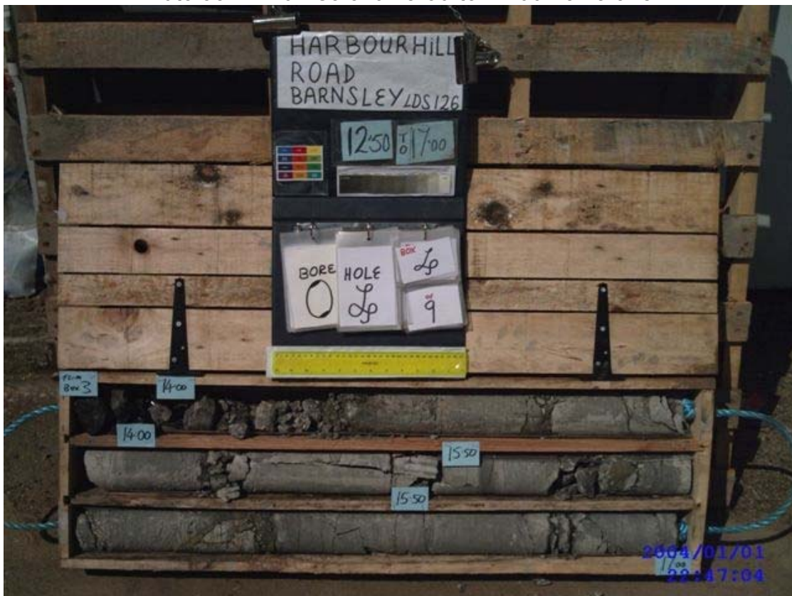
Plate 57 – BH04 Core run 12.50 to 17.00 Box 4 of 9
