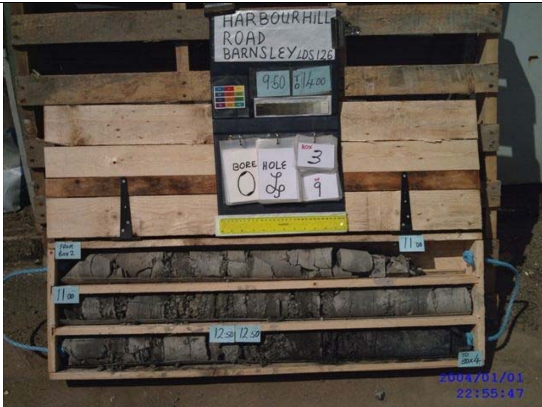
Plate 56 – BH04 Core run 9.50 to 14.00 Box 3 of 9
