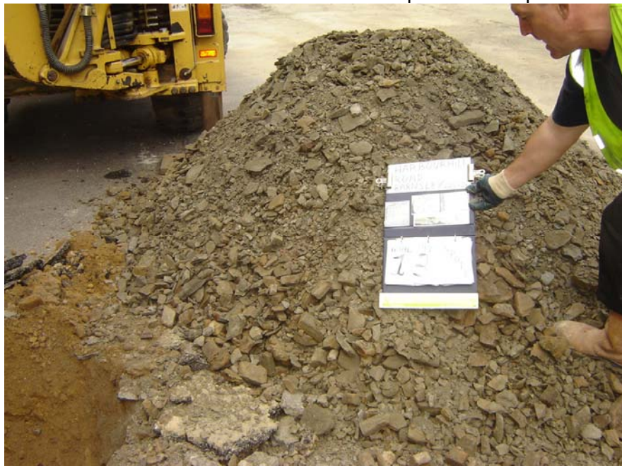
Plate 26 – Bedrock recovered as sandy gravelly cobbles of MUDSTONE.
