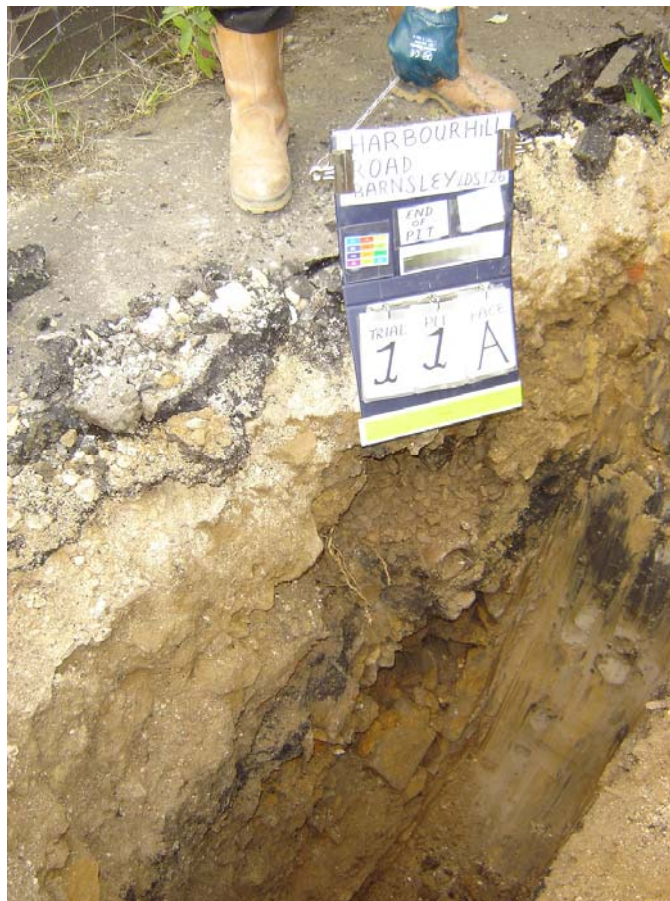
Plate 20 – Made ground was commonly above rockhead.
