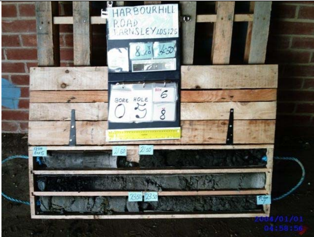
Plate 68 – BH05 Core Run 18.50 to 24.50 Box 6 of 8
