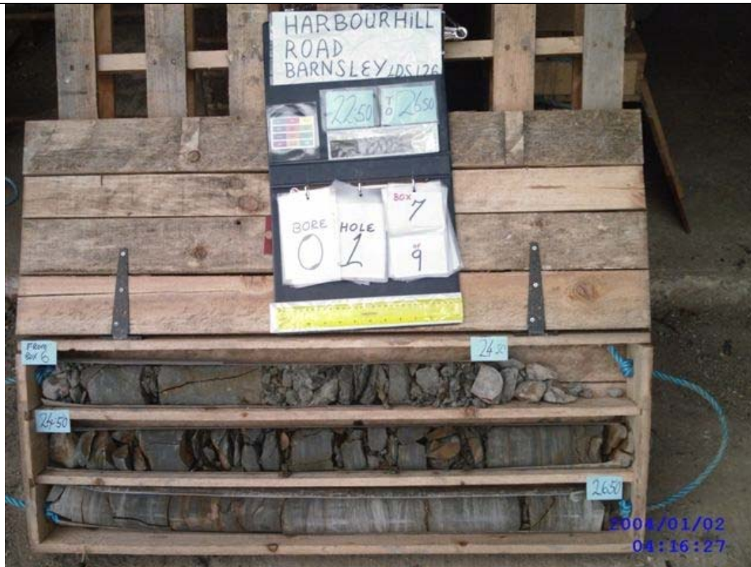
Plate 34 – BH01 Core Run 20.50 to 24.50 Box 7 of 9
