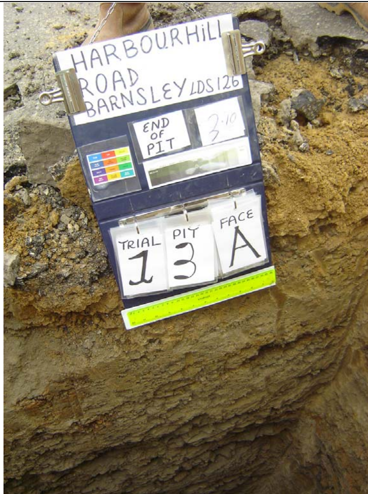
Plate 25 – Near surface rockhead Trial Pit 13. The pit was complete at 3.10m bgL.
