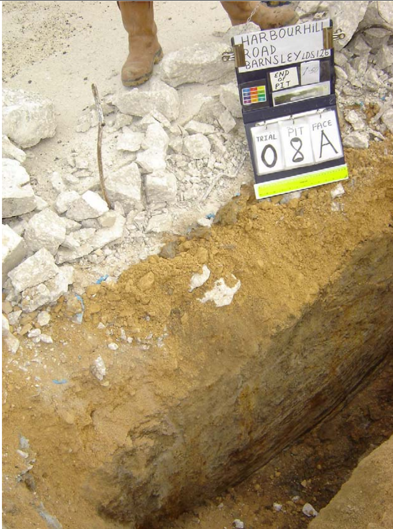
Plate 27 – Near surface rockhead Trial Pit 08. The pit was complete at 1.50m bgL.
