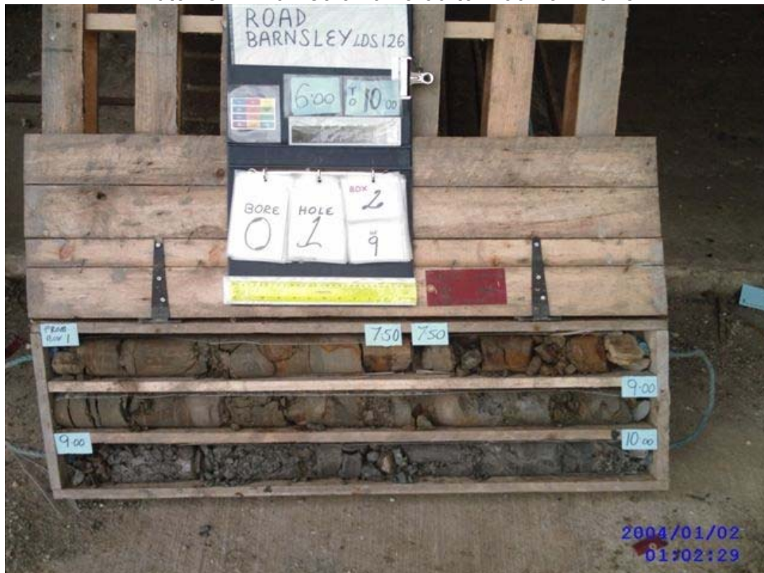
Plate 29 – BH01 Core Run 6.00 to 10.00 Box 2 of 9
