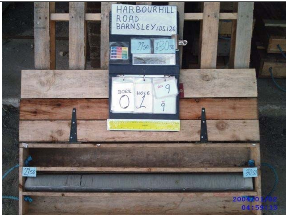
Plate 36 – BH01 Core Run 29.50 to 30.50 Box 9 of 9
