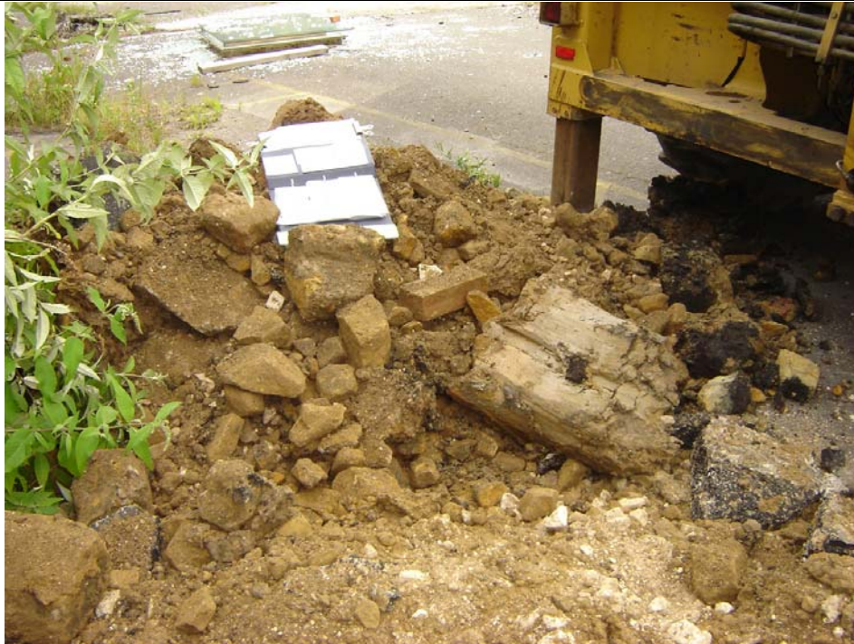
Plate 19 – Trial Pit 11 Made ground from faces A and D angular cobbles and boulders of sandstone and rare concrete to 1.90m bgL.
