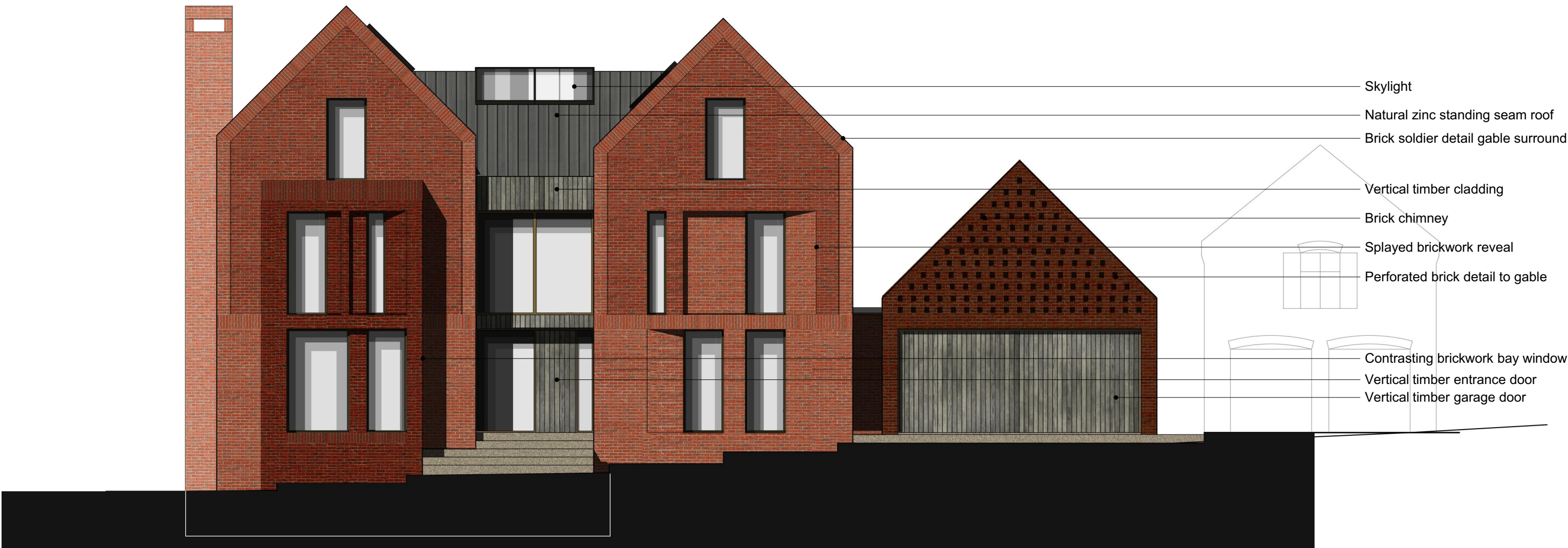
N 1:100 North Elevation (Coloured)
