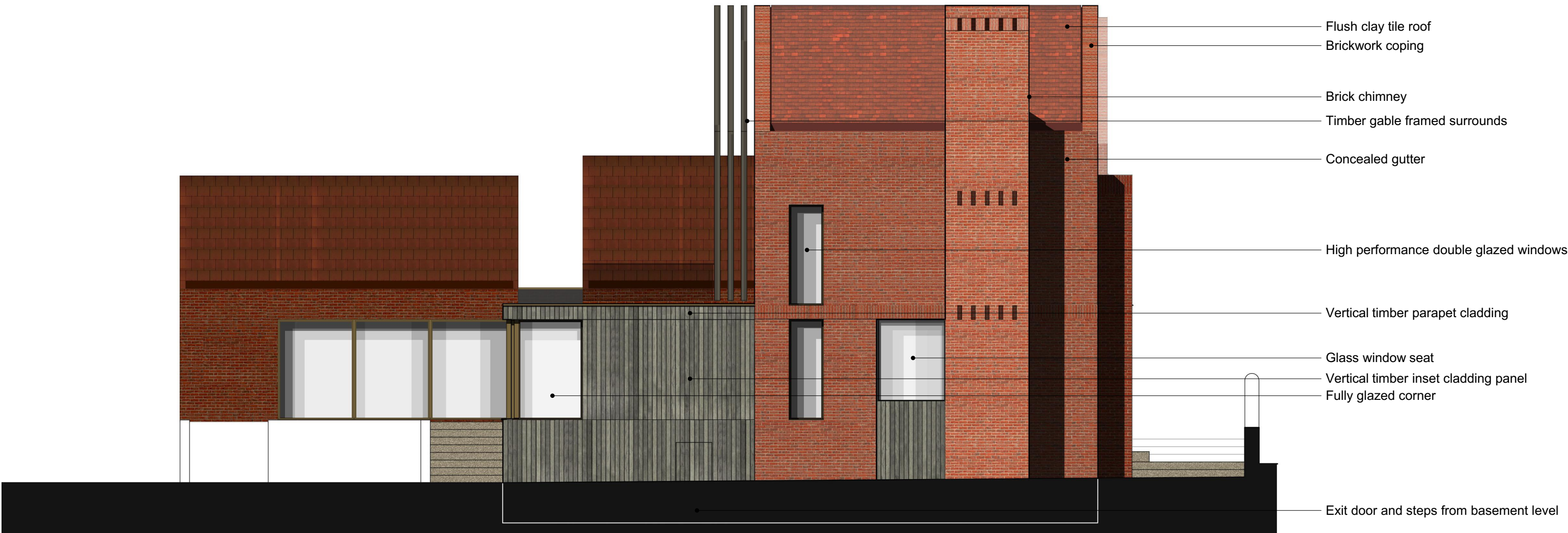
E 1:100 East Elevation (Coloured)
