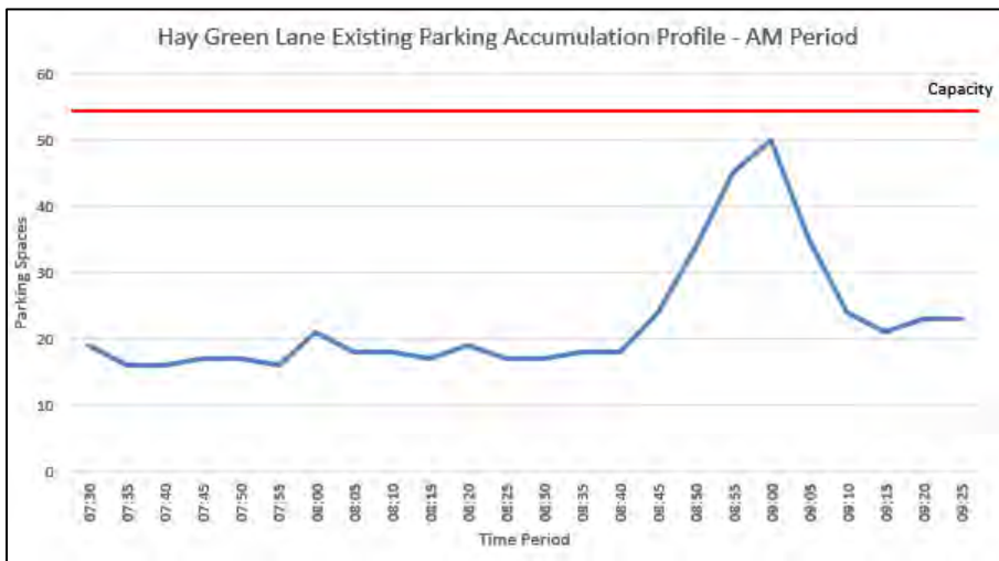
Image 2.15 Hay Green Lane Parking Accumulation – AM
