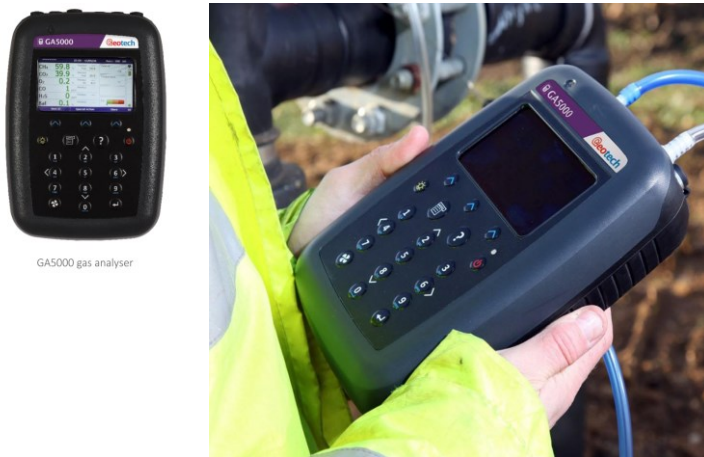
Fig 7 – Earth Tech’s Geotechnical Instruments GA5000 sampling system used at Hill End Farm, Hill End Road, Mapplewell, S75 6DU
