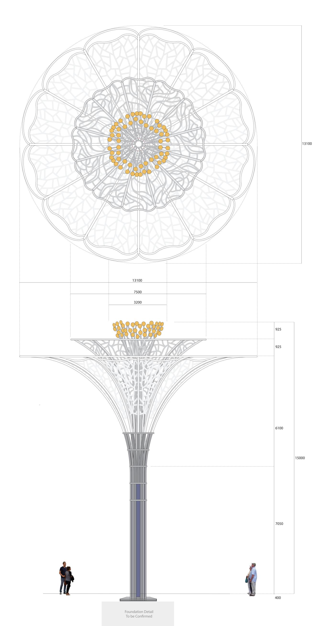
Three Super Structures are proposed for SEAM constructed in mild steel with protective decorative finishes with the central one 15 metres tall and the outer two 12 metres tail. The 'Yorkshire Rose' structure would create an organic flower bloom canopy with patterned steelwork that mirrors various weave threads, coal mining seams, the veins of white rose petals and stamens.
