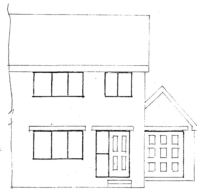
EXISTING FRONT ELEVATION
