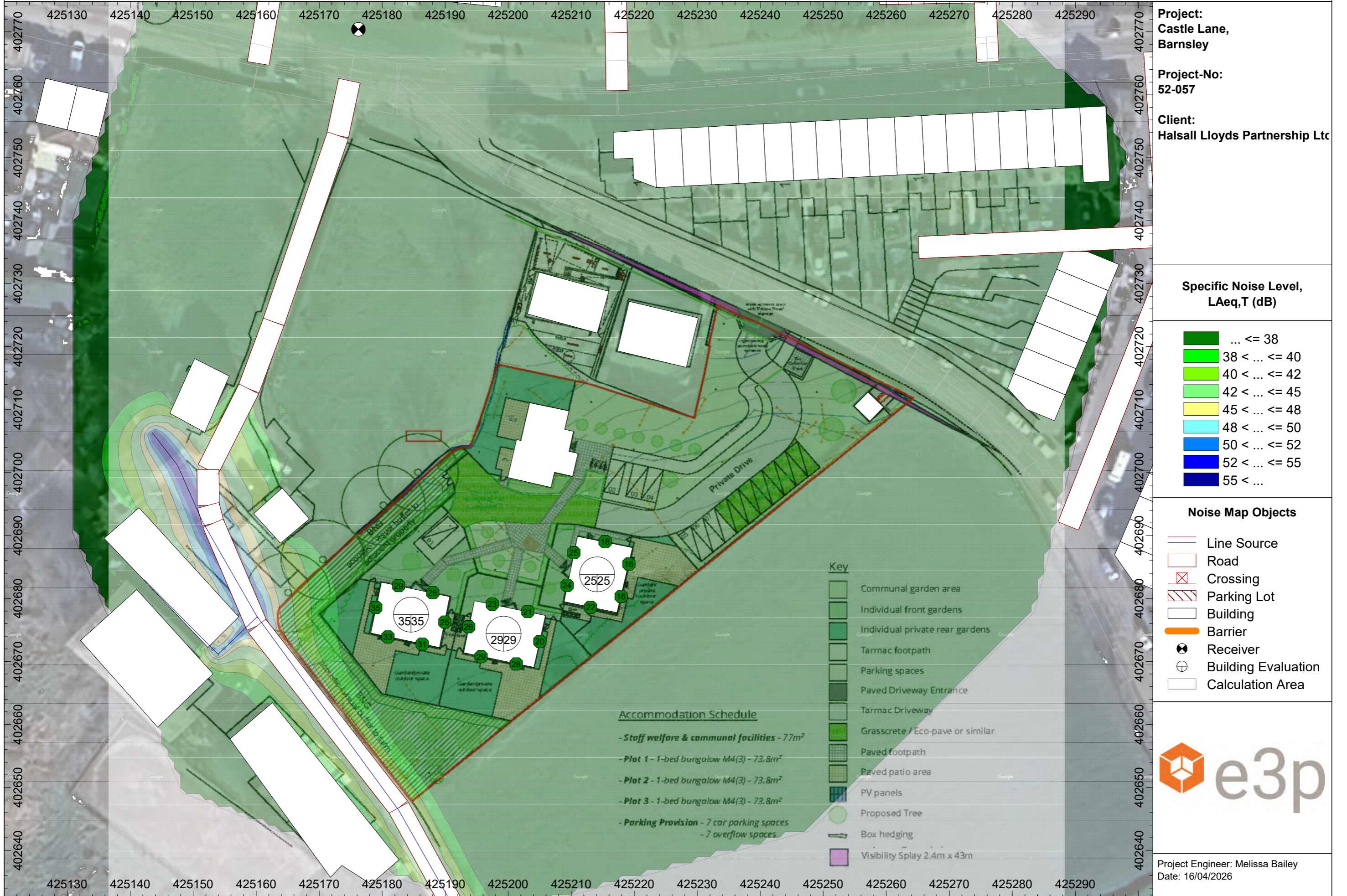
Figure 7 - Daytime Grid Noise Map (BS 4142) - Calculated at 1.5m above ground level
