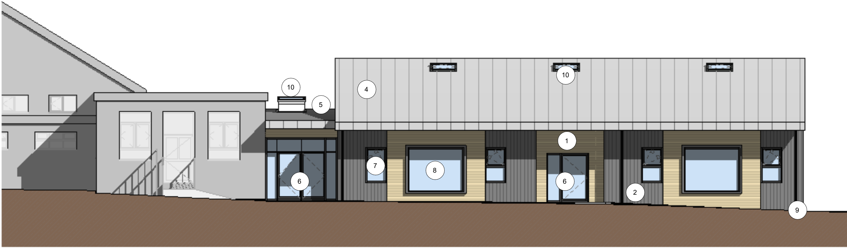
Proposed Front Elevation A 1 : 100
