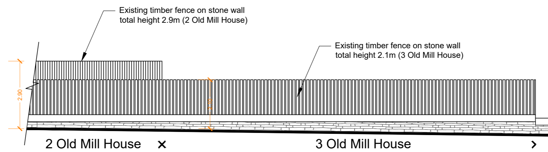
AS EXISTING REAR ELEVATION 1:100
