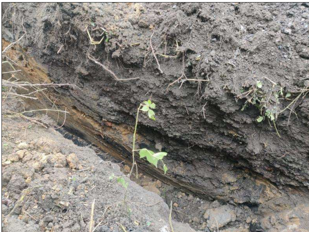
Photo 8: TP03 – Darker coloured backfill material with fragments of brick (adit 16) within the light brown natural strata.
