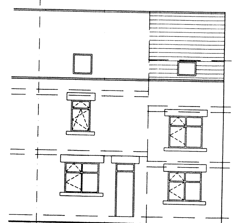
EXISTING FRONT ELEVATION
