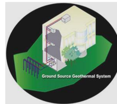
Ground Source Heat Pump Installation
