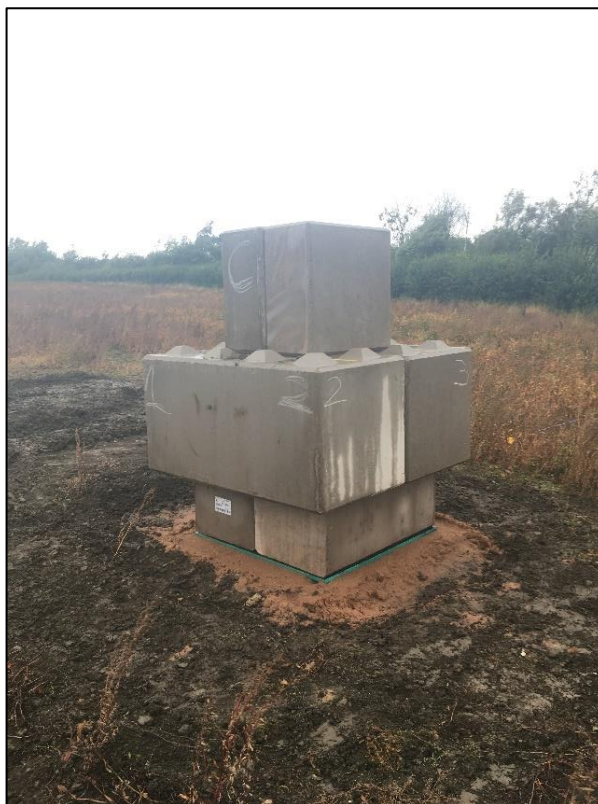
Plate F: Site example of the constructed Maintained Load Test.
