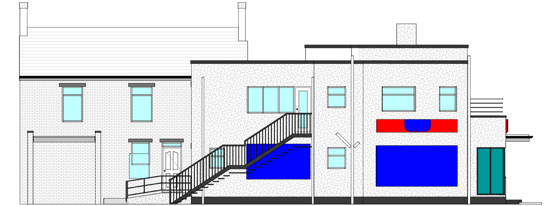
4 -Proposed Left Side Elevation 1 : 100
