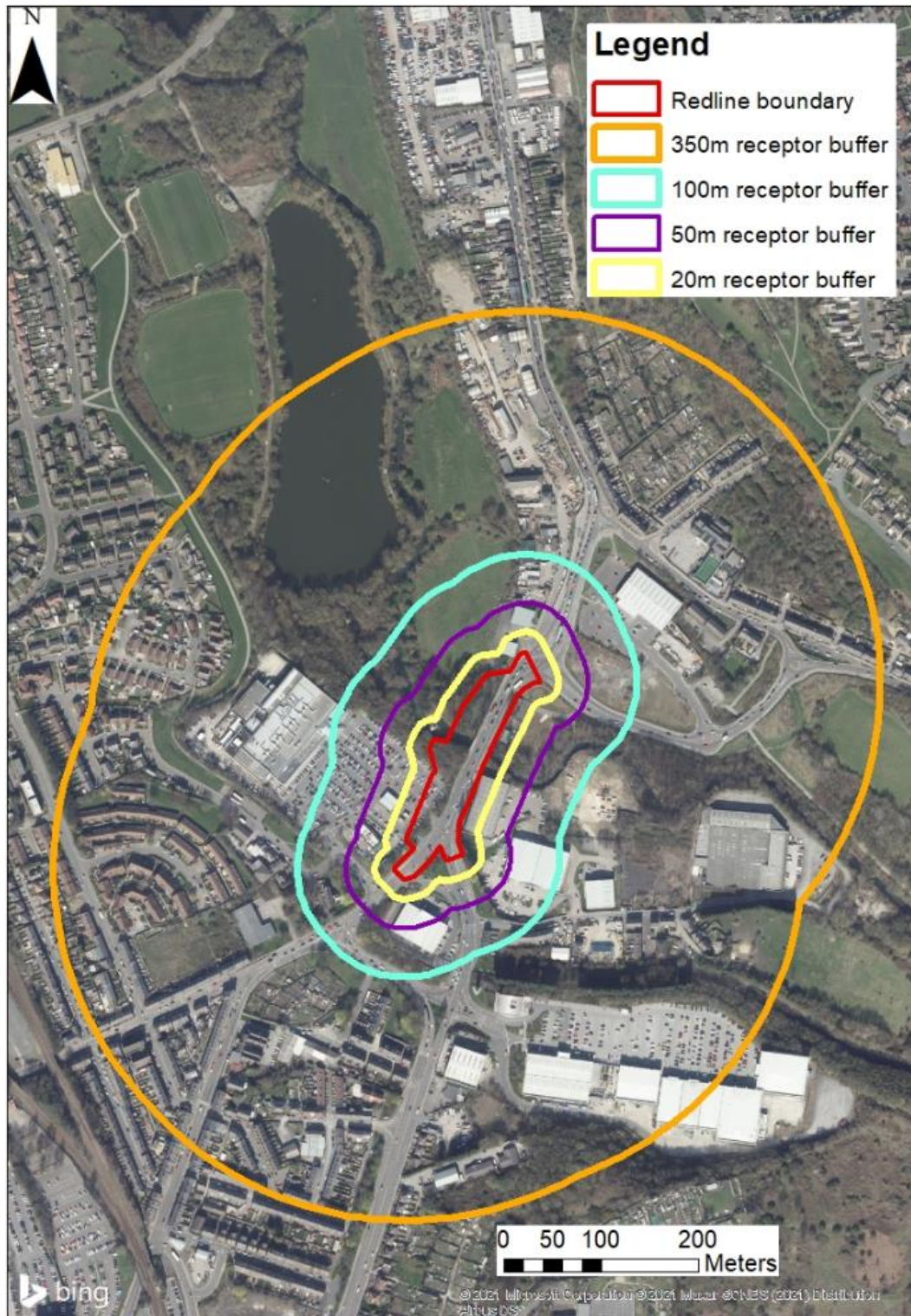
Figure 5: Construction dust buffers
