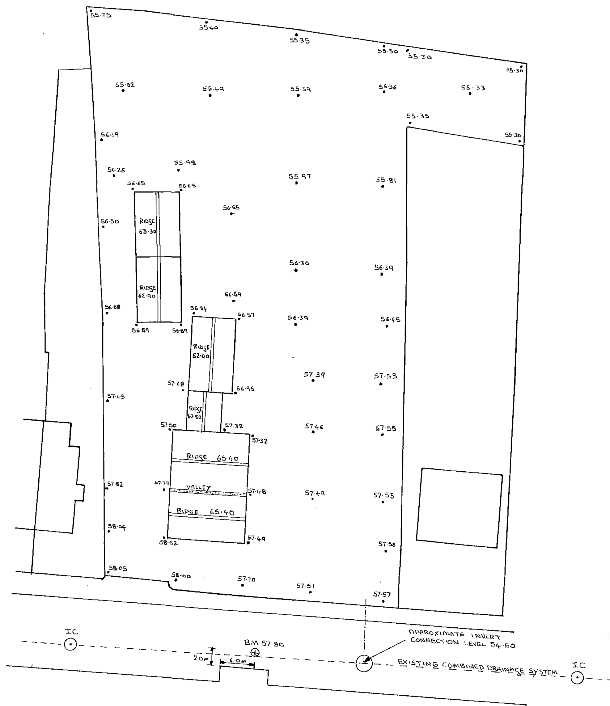
EXISTING LEVELS SURVEY SCALE 1:250
