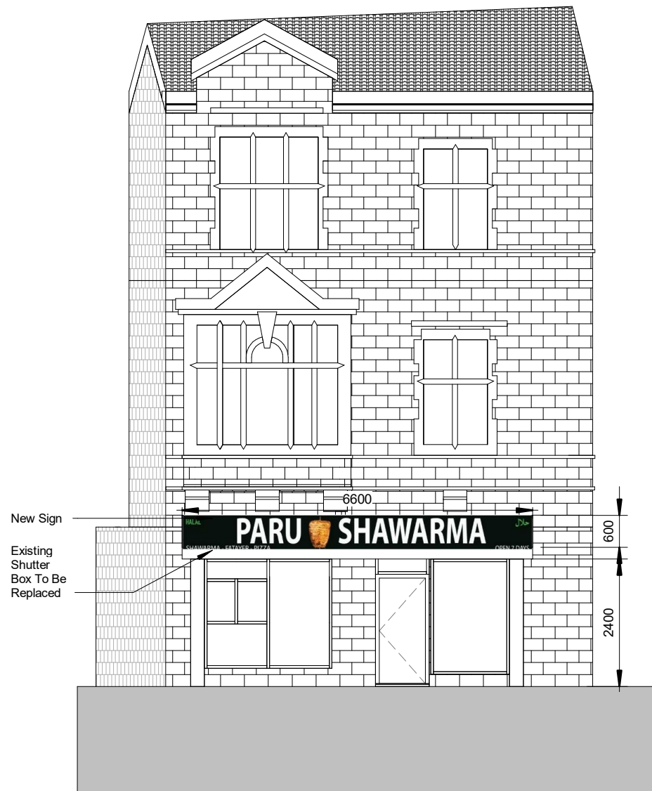
Existing Front Elevation 1 : 100
