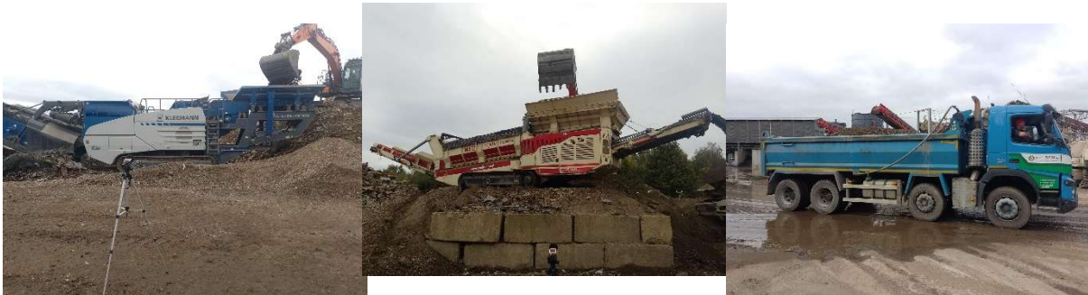
Pictures 1 – 3 (left to right) Kleeman mobile crusher/MDS M412 mobile trommel/HGV
