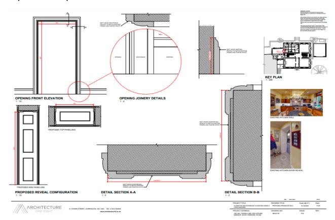
The applicant is seeking approval to create an opening between the kitchen and the Garden room. The materials used will be a soft wood opening reveal with raised and fielded panels. Top and side panelling profile to match existing, primed and painted white.
