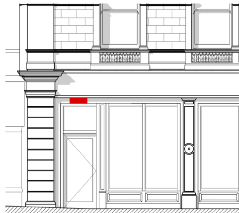
Street level luminaire - entrance
