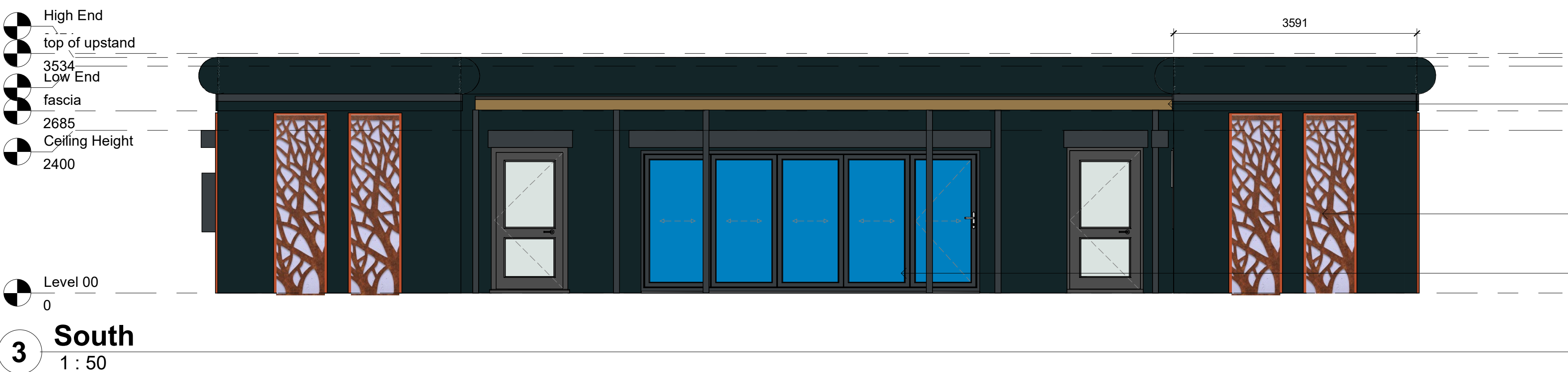
TBC - Retractable canopy, example above Bespoke corten steel feature panels Bi-fold doors to open/play area
