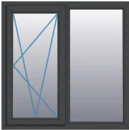
Inward opening style windows (to west elevation)
