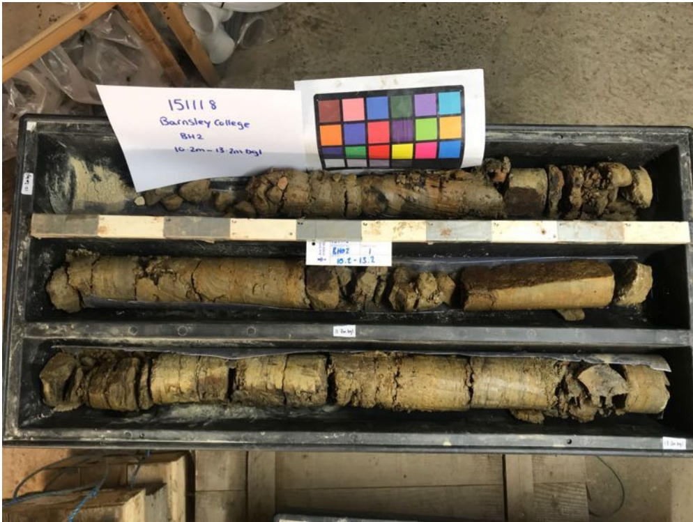
Plate 3: BH2 - 10.2m -13.2m bgl
